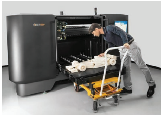
A large format 3-D printer for creating bigger products.
