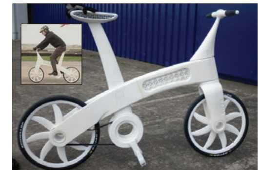
A 3-D-printed bicycle is fully functional by the time it emerges from the printer.
