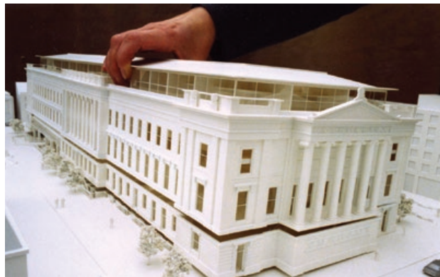
Model of a building created using a 3-D printer.
